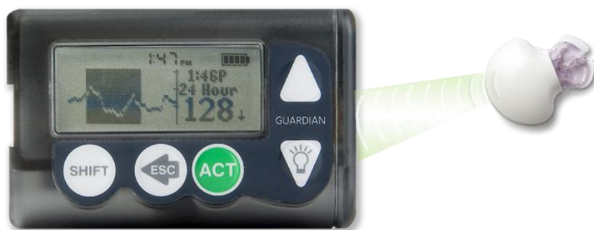
Fig. 3: Guardian ® REAL-Time (Medtronic) for continuous Glucose monitoring. The small sensor measures the glucose in the interstitial tissue (enzymatic reaction by using glucose oxidase). The data's transferred with a transmitter to the monitor (radio transmission).
